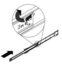
7 Hang the hooks of the rails on the rack holes and if necessary, secure with screws.
